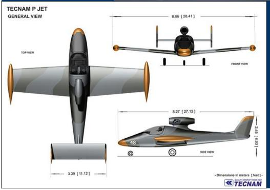
'P JET' cabin will be available both pressurized and non-pressurized, for use with an airframe integrated oxygen system.
