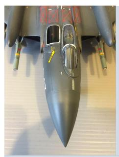
On the FAW.1 version the Observer's Cockpit was covered by a solid metal hatch (with a very small window) flush with the fuselage surface. On the later FAW.2 the hatch was raised slightly to give the observer more headroom, and was a frangible Perspex cover that the observer could eject through. Generally these were painted black on the inside in service, however XP924 currently flying in the UK has this left clear – presumably to make the ride less claustrophobic for any passenger.
