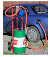
Putting a "big-ar\*e" fuel filter on my hand pump set up was one of the best pieces of advice that I got. I used my new set up to fuel my car for a while, the photo (right) shows some of the rubbish that the filter removed. By the time my fuel trolley got to the airfield it was perfectly clean. As the fuel drums had been used for fuel quite recently I hadn't rinsed them well. After
