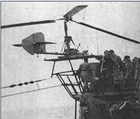
A Focke Achgelis Fa-330 Bachstelze (Wagtail) preparing to launch from a U-boat conning tower. Source: http://uboat.net/technical/bachstelze.htm , no attribution listed.
