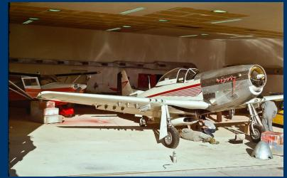
ZK-CCG being stripped of paint after arrival in the USA.
