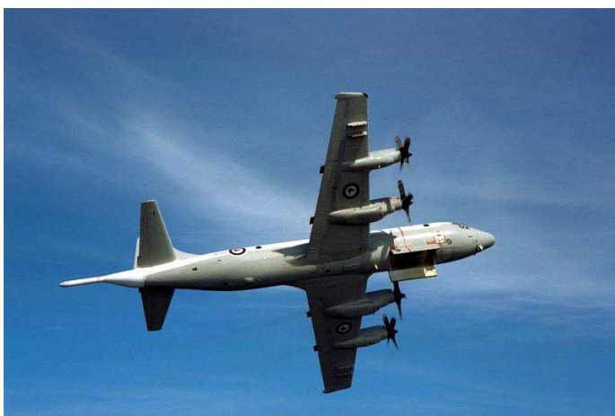
RNZAF Orion NZ4203 banks away from the camera. This was shortly after the conversion to P-3K standard, note the new IRSD turret under the nose, lack of the Searchlight pod, and the early white/light grey colour scheme.
