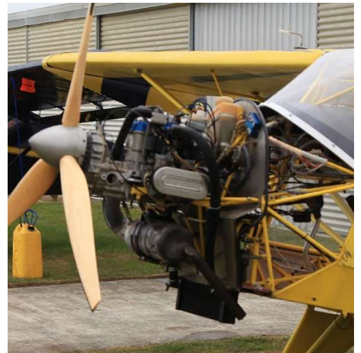
Above, Mike Godfrey's Kitfox ZK-KIV at the Rangiora Airfield open day, showing the high standard of workmanship on these aircraft. The Rotax 582 is shown in detail, Right
