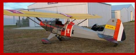
YES, THE POBER PATHFINDER IS FOR SALE (PIXIE IS NOT RIGHT) VW 1730 CC DUAL PORT HEAD All chrome molly fuselage and spruce wings. Only 120HRS on Airframe and much less on the latest engine. Easy to fly and reliable.
