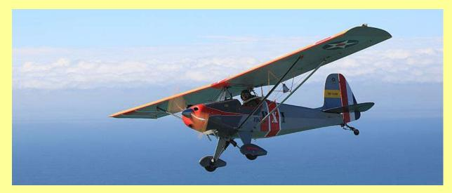
VW 1730 CC DUAL PORT HEAD All chrome molly fuselage and spruce wings. Only 120HRS on Airframe and much less on the latest engine. Easy to fly and reliable.
