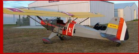
YES THE POBER PATHFINDER IS FOR SALE (PIXIE IS NOT RIGHT) VW 1730 CC DUAL PORT HEAD All chrome molly fuselage and spruce wings. Only 120HRS on Airframe and much less on the latest engine. Easy to fly and reliable.
