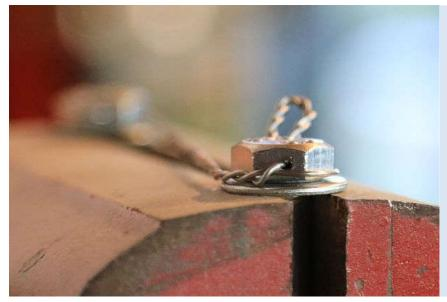
Left, another view on the 'two-bolt' demonstration. Note how the end coming around the bolt head goes under the end exiting the bolt head hole. This ensures that the wire will not vibrate over the top of the bolt head and come loose.
