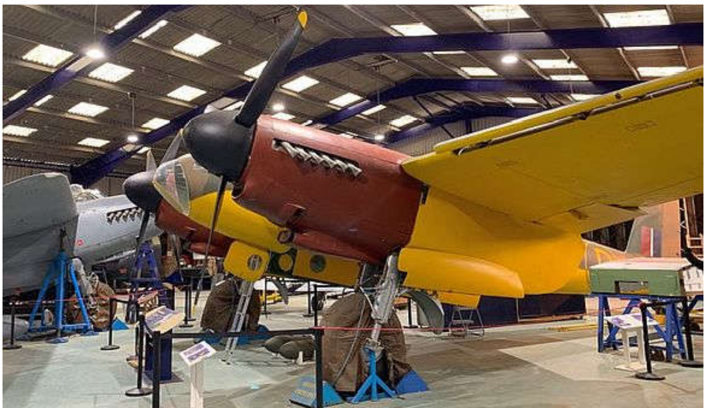
Below, the DH 98 Mosquito first prototype, complete with leading edge slats (which never made it to production) and the later two-stage Merlins, showing how it was used to test later developments.
